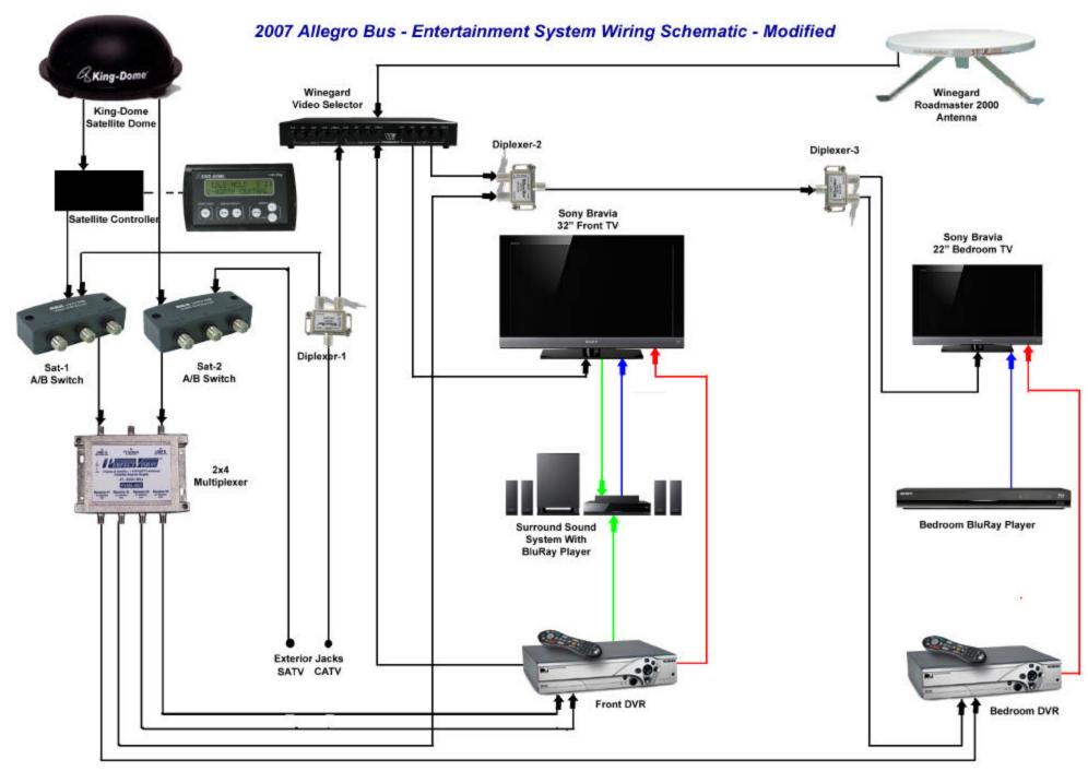
Black Lines = RG-6 Quad Shielded Coax Red Lines = Component Video plus Audio Blue Lines = HDMI Audio/Video Green Lines = Stereo Audio
